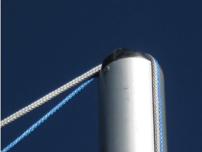
Both the halyard and depowering line pass through the mast cap
