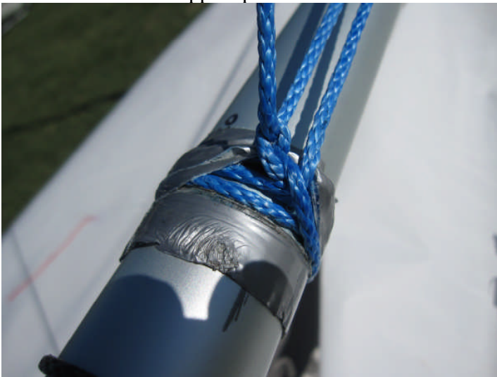
A very small bowline is tied at the bitter end of the depowering line (at the free end of a rolling hitch)
