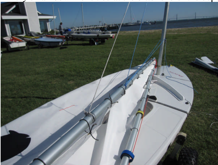
The depowering line is led around the mast, back through the very small bowline and then with the halyard up through the mast cap
