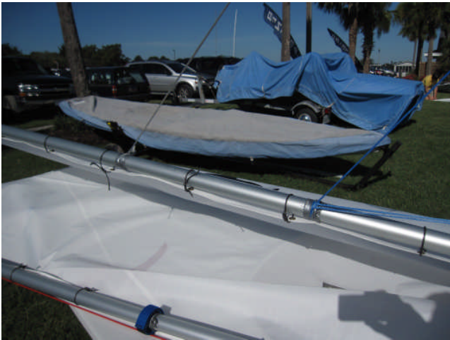
Regular halyard (gray color) tied in normal position and depowering line (blue line) tied down as far as 20-inches lower on the upper spar
