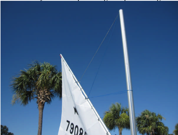
Both the halyard and depowering line are hoisted simultaneously and the depowering line loops around the mast and rises and adjusts automatically
