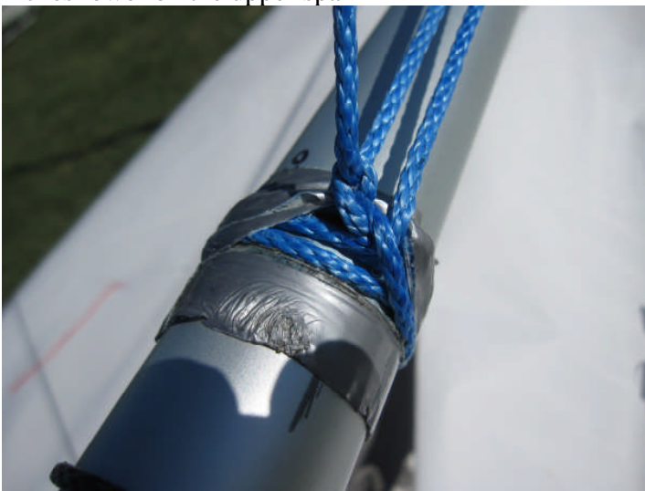
A very small bowline is tied at the bitter end of the depowering line (at the free end of a rolling hitch)
