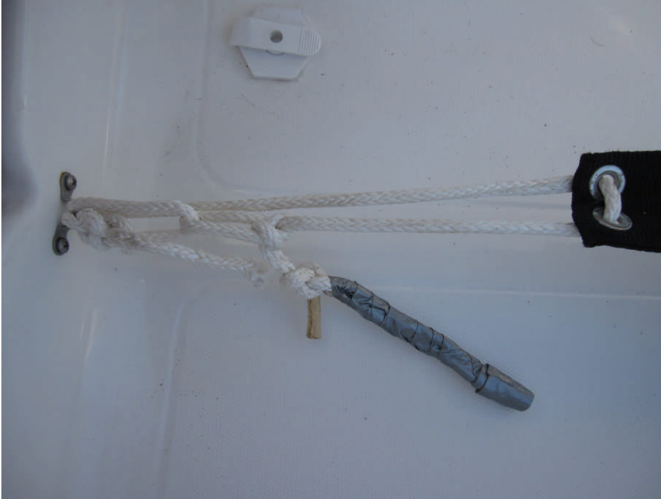
Grommets added to end of hiking strap and simple tensioning line used to create an adjustable hiking strap
