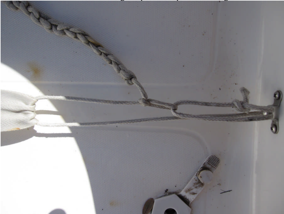
Same version but with no grommets added to hiking strap
