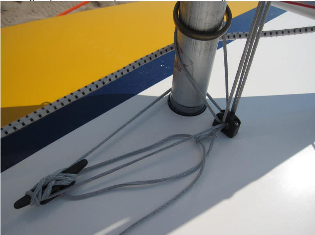
Beginning of an adjustable vang with one purchase tied in near the deck bullseye (the deck cleat is used as a fixed point to develop 3:1 mechanical advantage)
