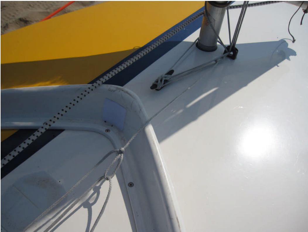
Additional purchases are added as the running end of the halyard is led back to the cockpit
