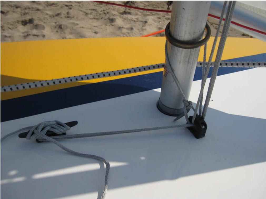
Standard vang with tail of main halyard starting with the running end tied to the deck bullseye with a bowline, passed over the top of the vang, back through the bullseye and then to the deck cleat. A 2:1 mechanical advantage is produced but no purchases are tied in the vang line.
